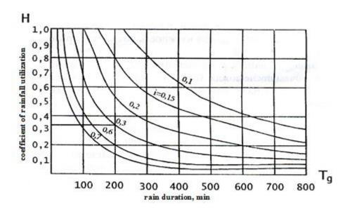
Figure 2. Nomogram for determining utilization rate of rainfall.
