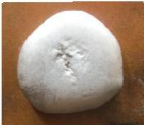
Figure 2b:- Photographs of Sn 96.5-x Ag 3.5 Bi x molten alloys on Cu substrate in air
