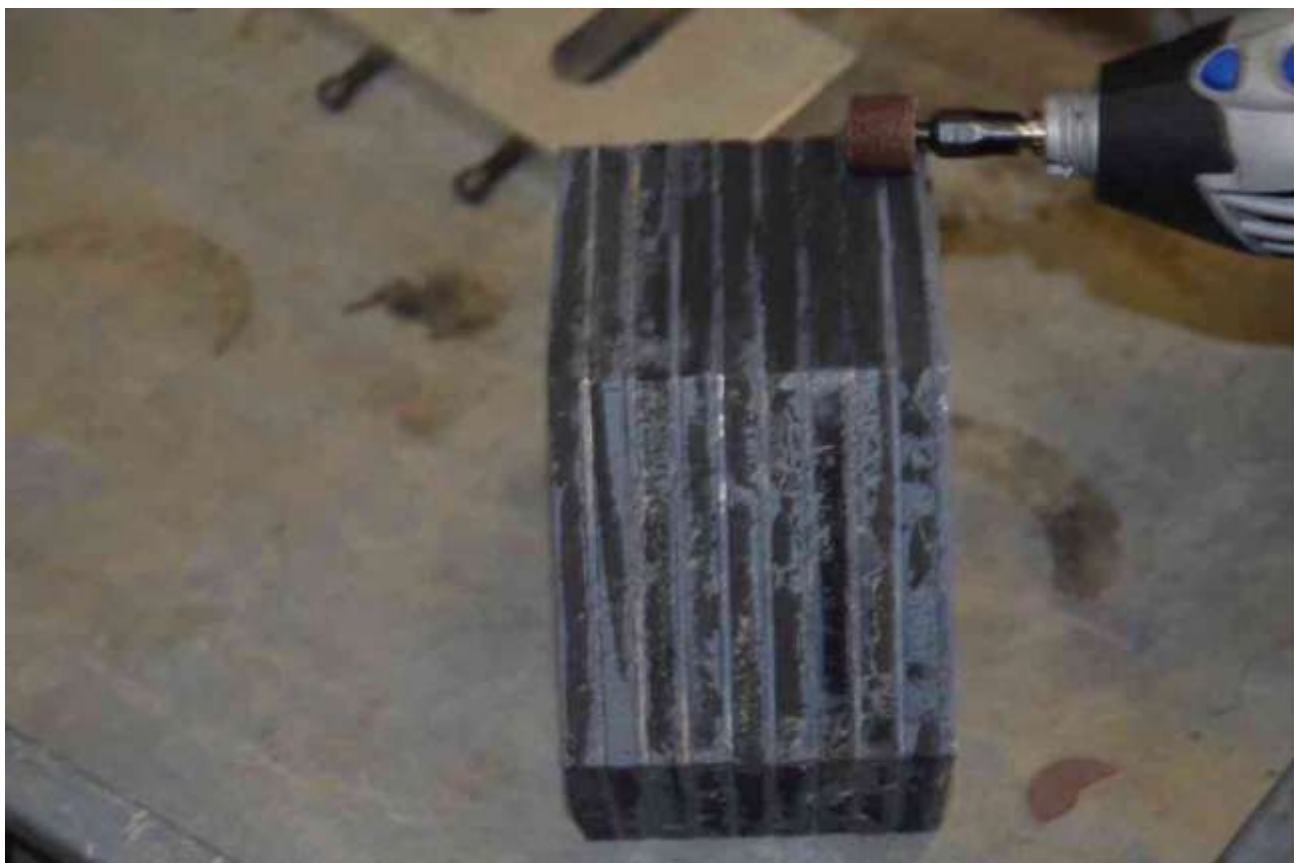
Figure 4: Inner High Damping Rubber Bearing Layers
