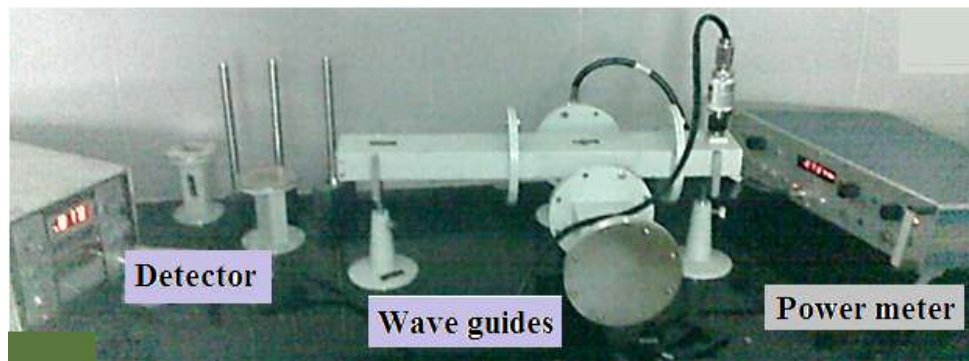
Figure 3 Microwave set up showing the arrangement of wave guide with power meter and the detector for the reflected wave
