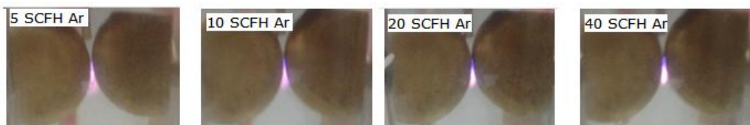
Fig. 3: photograph of GAD plasma for different argon gas flow rate at 2.7 kV discharge voltage.
