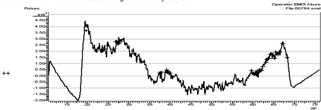
Fig.1: XRD for as-deposited \text{TiO}_2/\text{MnO} Thin Film
