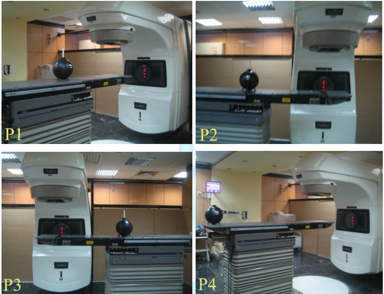
Fig. 2. Linac, LB 6411 polyethylene sphere, and the sites where the neutron doses were measured. Five TLD pairs are located in the center of LB 6411 polyethylene sphere.
