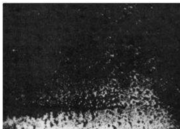
Fig. 3 The optical micrograph of etch pits on the (111)A surface
