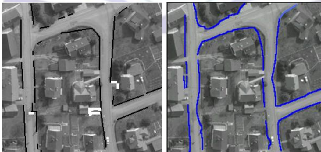
Fig 6: Experimental results. (a) Extracted straight lines grouped by ACA, and (b) detected roadsides overlaid on the filtered image of Fig. 2(a).
