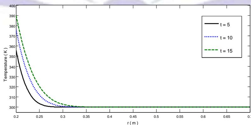
**Fig 2: Temperature distribution for  $t = 5, 10, 15(s)$ , heat flux  $Q_0 = 100J / sm^2$**
