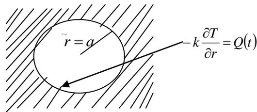
Fig.1: Geometry of infinite body with spherical cavity
