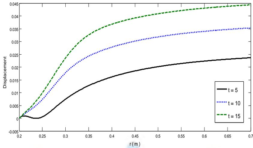
Fig 3: Radial Displacement for  $t=5,10,15(s)$ , heat flux  $Q_0 = 100 J / sm^2$
