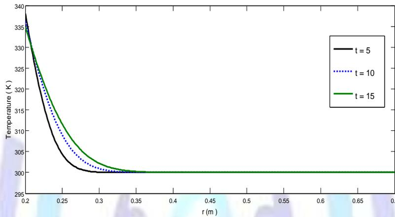
**Fig 6: Temperature distribution for  $t=5,10,15(s)$ , heat flux  $Q(t)=100t^{-\frac{1}{2}} J / sm^2$**
