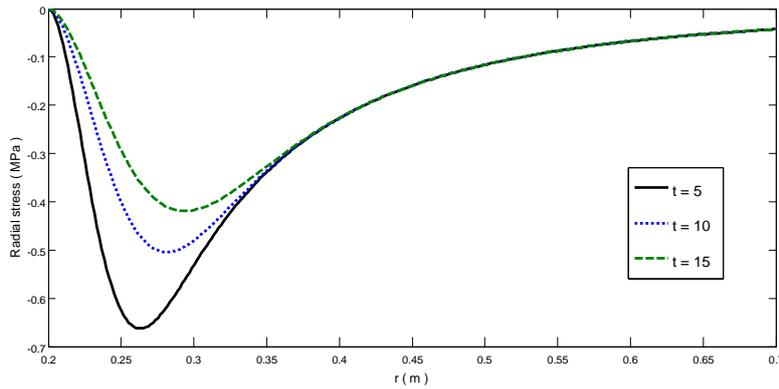
Fig 8: Radial stress distribution for for  $t=5,10,15(s)$ , heat flux  $Q(t)=100t^{-\frac{1}{2}} J / sm^2$
