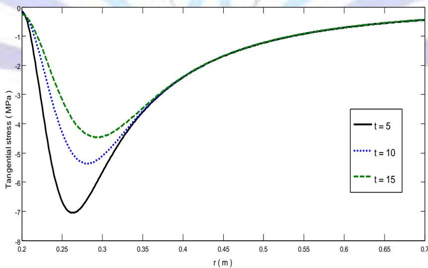
Figure 5 : Tangential Stress distribution for  $t=5,10,15(s)$ , heat flux  $Q_0 = 100 J / sm^2$
