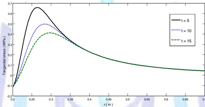
Fig 9: Tangential stress distribution for  $t=5,10,15(s)$ , heat flux  $Q(t)=100t^{-\frac{1}{2}} J / sm^2$
