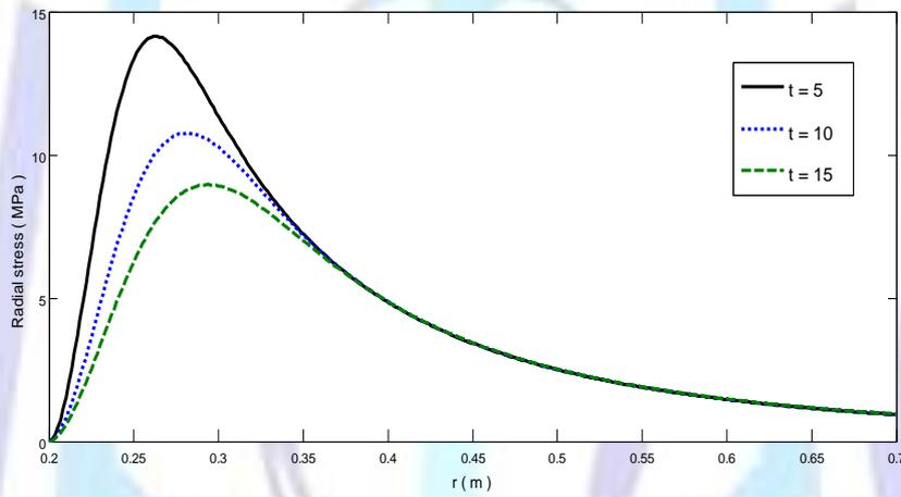
Fig 4: Radial stress distribution for  $t=5,10,15(s)$ , heat flux  $Q_0 = 100 J / sm^2$
