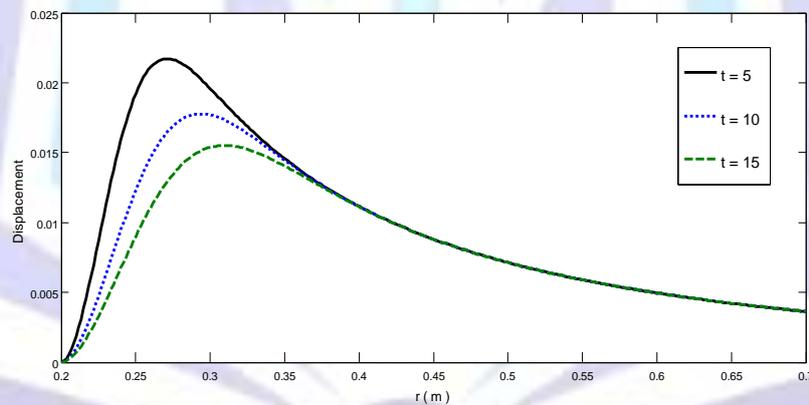
**Fig 7: Radial Displacement for  $t=5,10,15(s)$ , heat flux  $Q(t)=100t^{-\frac{1}{2}} J / sm^2$**
