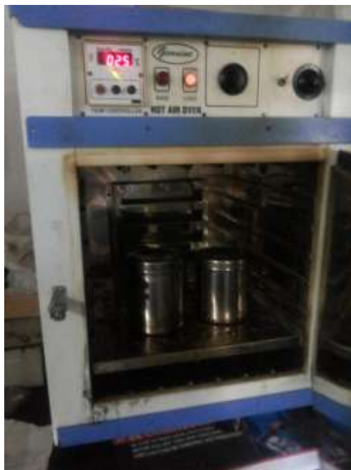
Fig 5: Picture of oven used for thermal aging of oils
