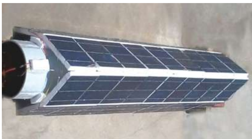
Fig. 5 Modified structure 100 Watts panel
