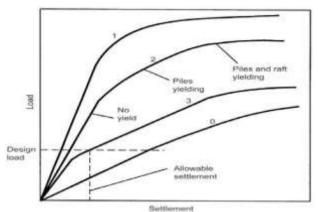
Figure 2 Load-settlement curves (Poulos, 2001)
