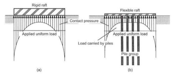
Figure 4 Distribution of contact pressure (a) rigid and (b) flexible rafts (Horikoshi & Randolph, 1998)
