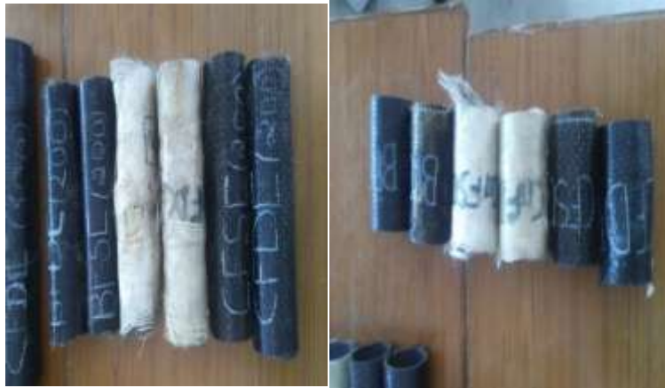
Fig. 1 Specimens wrapped circumferentially
