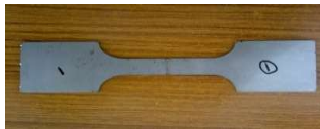
Fig. 1(b) . Photograph of a tensile specimen
