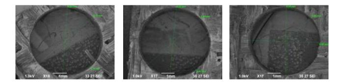
Fig 3: Microscopic picture of the composites for various drill speed of 1000, 2000 and 3000 rpm with constant feed rate of about 10 mm/min.
