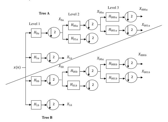
**Figure 6: Dual Tree Complex Wavelet Transform**
