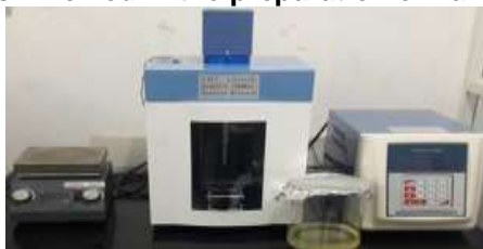
Fig.2 . Photograph of magnetic stirrer and ultrasonicator used in the preparation of nano-FR3 oil
