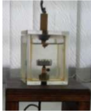
Fig.3. Photograph of test cell used for lightning impulse test
