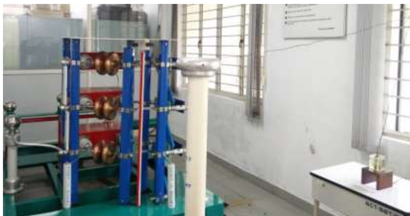
Fig. 5. Photograph of 3 Stage, 300 kV Lightning Impulse Generator connected to the test cell.
