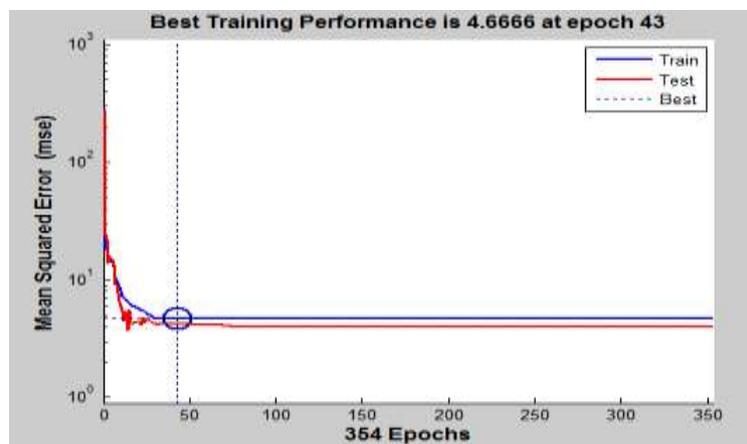
Fig. 18. Mean square error graph of BR method for process fault
