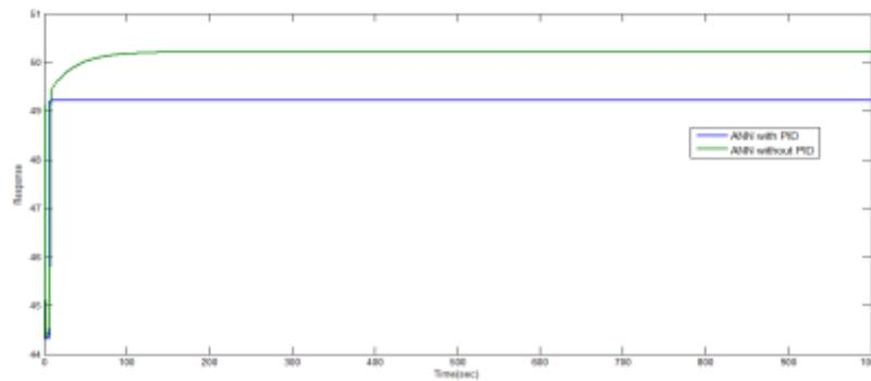
Fig. 17. Simulation results of BR method for sensor fault
