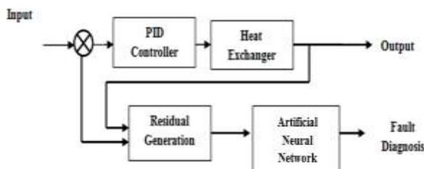
Fig. 6. Fault Detection using ANN
