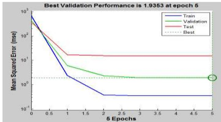
Fig. 9. Mean square error graph of LM method for sensor fault
