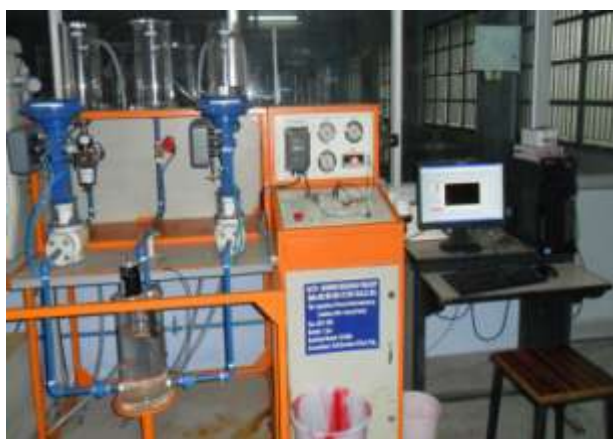
Figure 1 Real Time Experimental Setup of pH Neutralization Process
