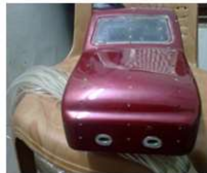
Fig 4. Location of base bleed in car and attachment Fig 5 Scaled model car in the wind tunnel Base Bleed
