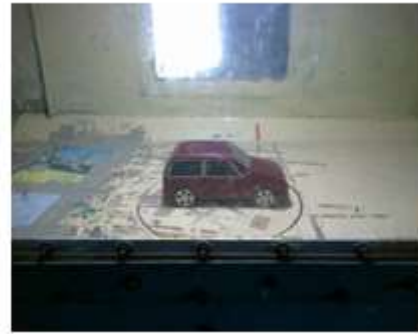
Fig.3 Scaled model car in the wind tunnel
