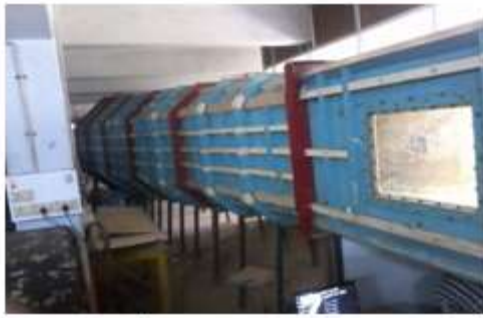
Fig.2 Subsonic closed-loop wind tunnel
