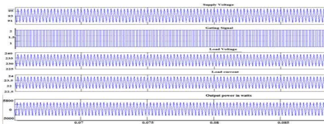
Fig 9: Output waveform of PV system with MPPT.
