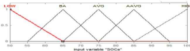
Fig 5: Input membership functions of  $\text{SoC}_e$
