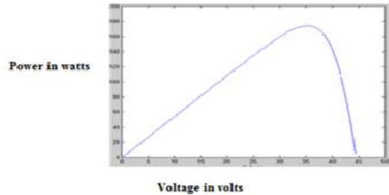
Fig 3: P-V characteristics of PV cell
