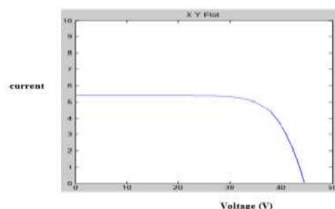
Fig 2: V-I characteristics of PV cell
