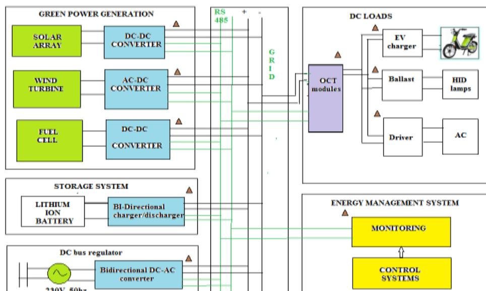
Fig 1: Block diagram of the proposed system
