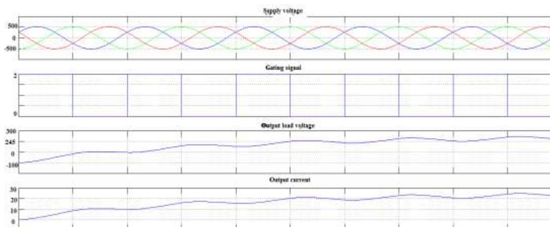
Fig 11: Output waveform of the wind energy conversion system.
