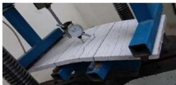
Figure1 Flexural test setup
