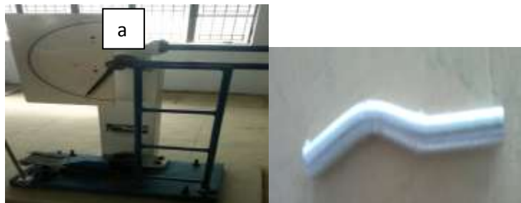
Fig 3.7 a) Impact tester , b.) specimen after test.
