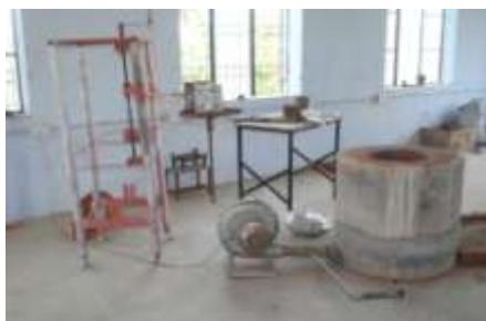
Fig 3.2 melt stir cast set-up
