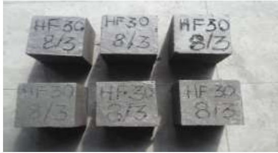
Fig 12: cube specimen before acid attack
