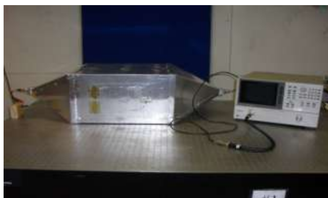
Figure 3: Experimental setup for characterizing the impedance of PIFA
