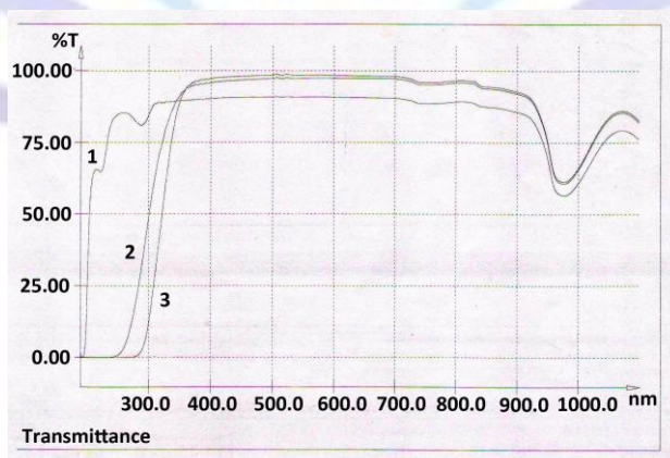
Fig 5: EAS of aqueous solution containing: 1- 1.0 mas.% PEG6000, 2- 1,0 mas.% sodium salt of succinic acid; 3- 1.0 mas.% PEG6000 and 1,0 mas.% of sodium salt of succinic acid
