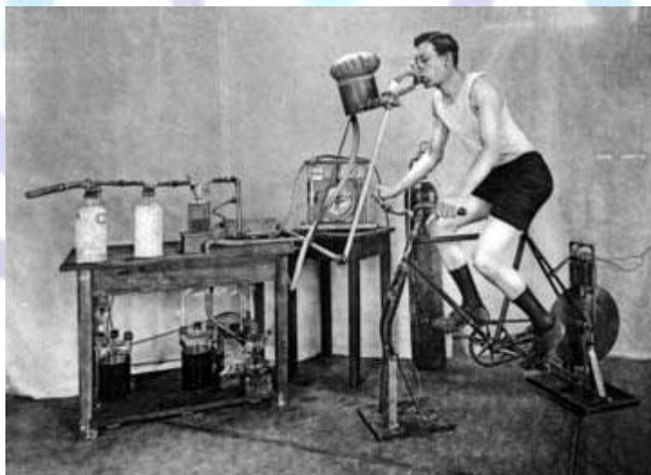
Original bicycle ergometer used in Benedict's experiments to assess exercise energy metabolism in the early 1900s
