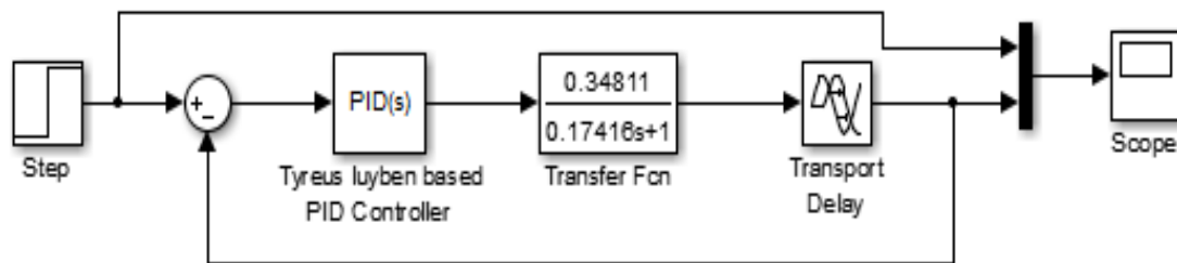
Fig 6: Simulink model for PID controller based on Tyreus Luyben
