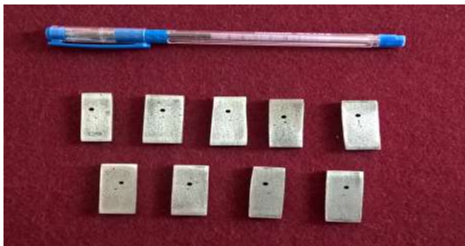
Fig:1 EDM Drilled Monel Alloy.
