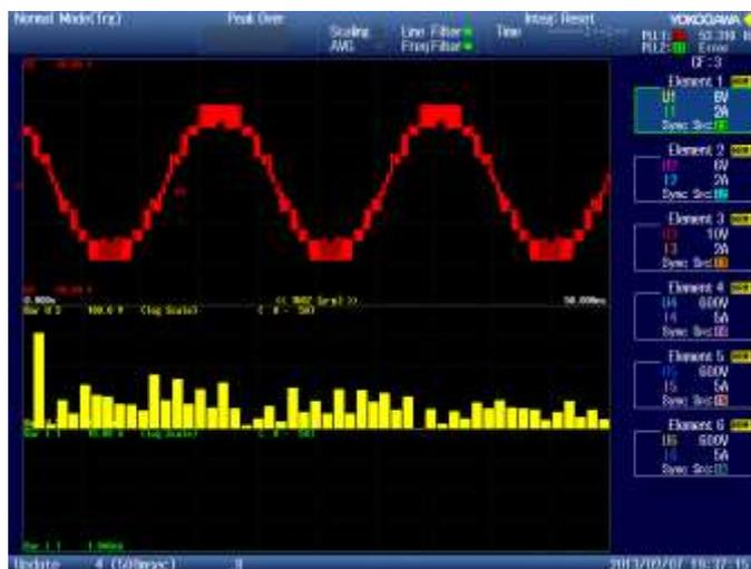
Fig 16. THD bar chart for thirteen level Inverter.
