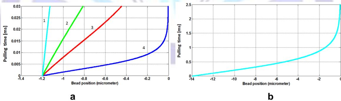
**Fig 5: a) Stretching processes of plasmid DNA molecule at initial position of  $r_0 = 1.2mm$  (90% of contour length) using laser beam with beam waist  $W_0 = 1mm$  and different peak intensities**
