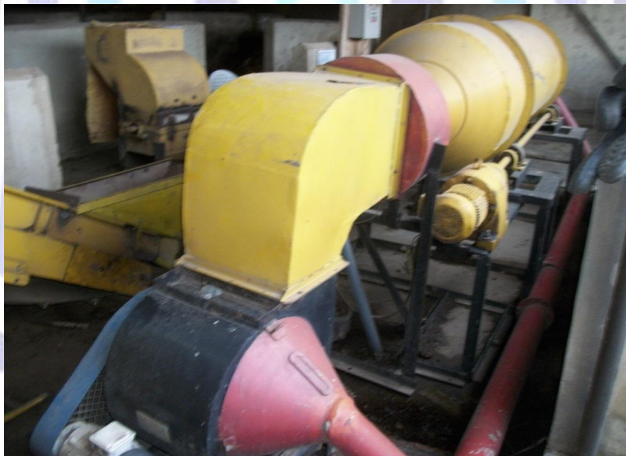
Figure 2. Artificial drying of compost by Electric Rotary Dryer(ERD) machine
