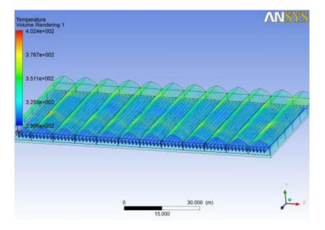
Figure 4. Temperature distribution indoor of the greenhouse.
