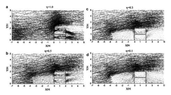
Figure 1 Effect of a porous media on natural ventilation, over high porosity by (a) to less porous (d) [9].
