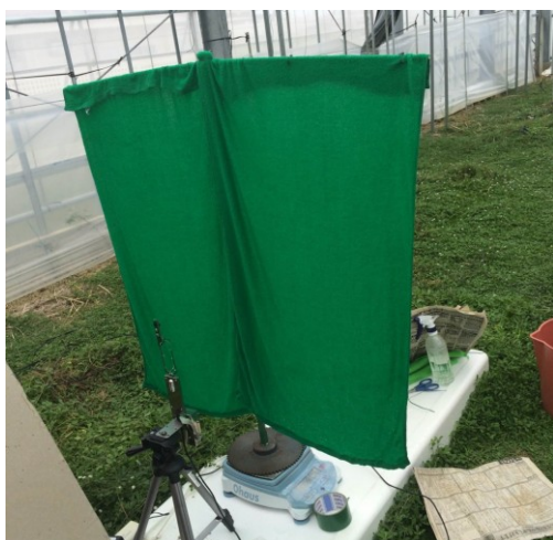
Fig. 3a. Artificial leaf made of towel sheet on the weighing machine with one sensor unit and hidden unit on the other side.
