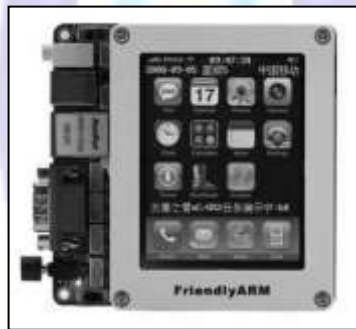
Figure 1 – FriendlyARM Mini2440 Development Board
