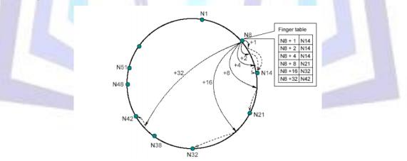
Figure 1. Chord network topography. The successor of the node  $N_8$  by 1, 2 and 4 steps is the node  $N_{14}$ , by 8 steps is the node  $N_{21}$  and so on.
