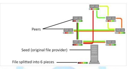
Figure 2. Simplified example of file's pieces destribution using Bittorrent protocol.
