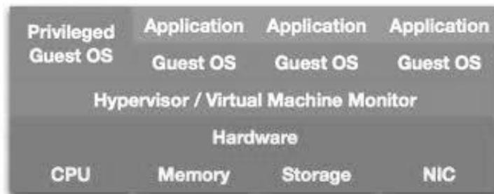
**Figure-3 Para Virtual Machine Server Virtualization**
