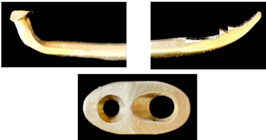
Figure 5 Coupling plate, knobbed headend and leading blunt barbed end.
