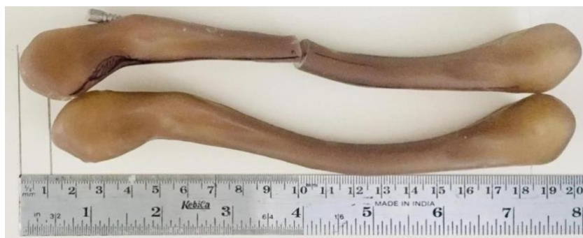
Figure 15 Lengthening of the clavicle upon application of a rigid intramedullary CRISP-G in a 5/10 station osteotomy of a Sawbone® clavicle.
