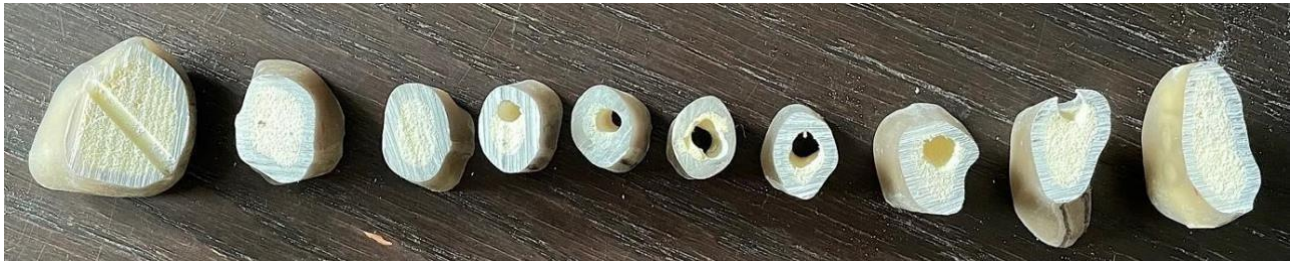
Figure 6. Note changing cross-sectional profile of the segments and eccentric holes left after the removal of an intramedullary implant inserted retrograde in a Sawbone®
