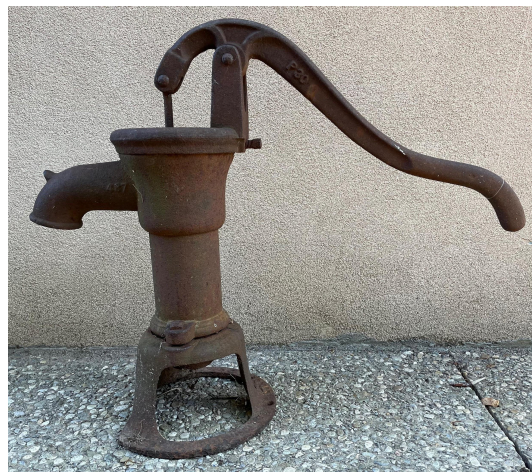
Figure 16. Kitchen water pump.
