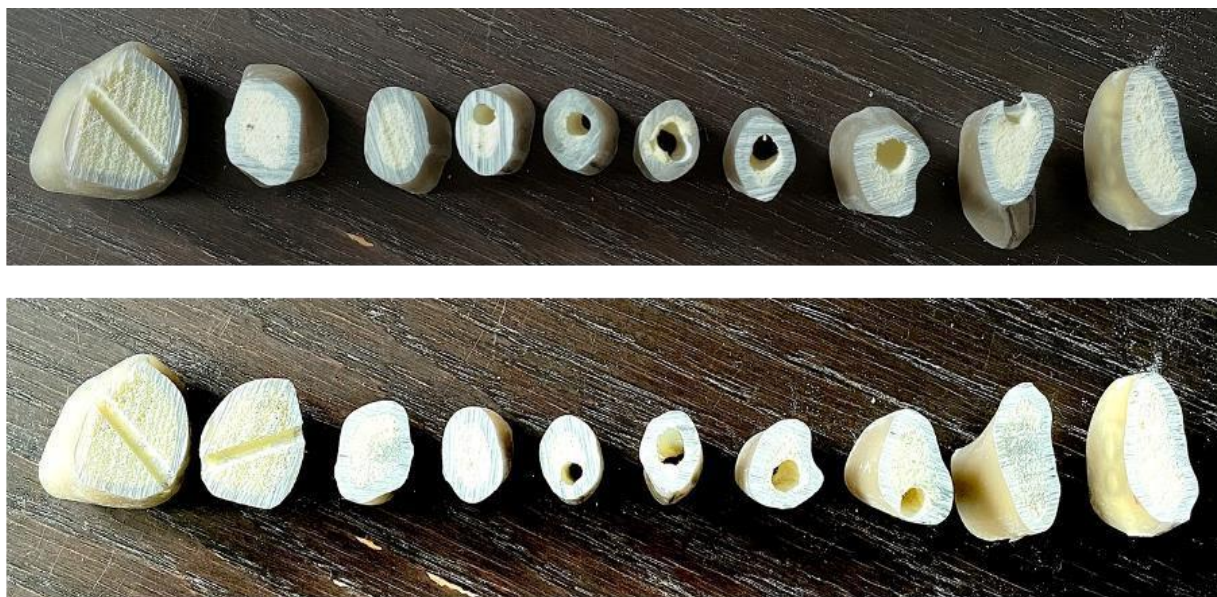
Figure 3. Highly variable shapes and sizes of the cross-sections of the same Sawbone®, viewed from both sides of the same section of the diaphysis, on the left is the sternal end. The holes are remnant of an intramedullary implant inserted from the acromial to the sternal end.
