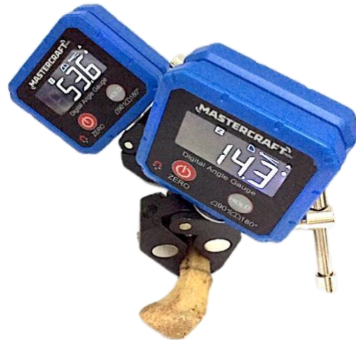
Figure 9. Digital goniometer devices are applied at the proximal and distal parts of the diaphysis of a cadaveric clavicle, which has a torsion angle of 39.3 degrees.
