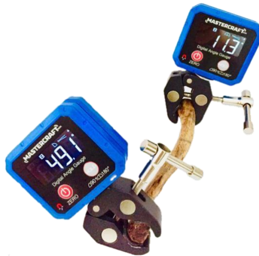
Figure 10. Digital goniometer measurements taken at the furthest sternal and acromial ends of a right cadaveric clavicle, showing a version angle of 37.8 degrees.
