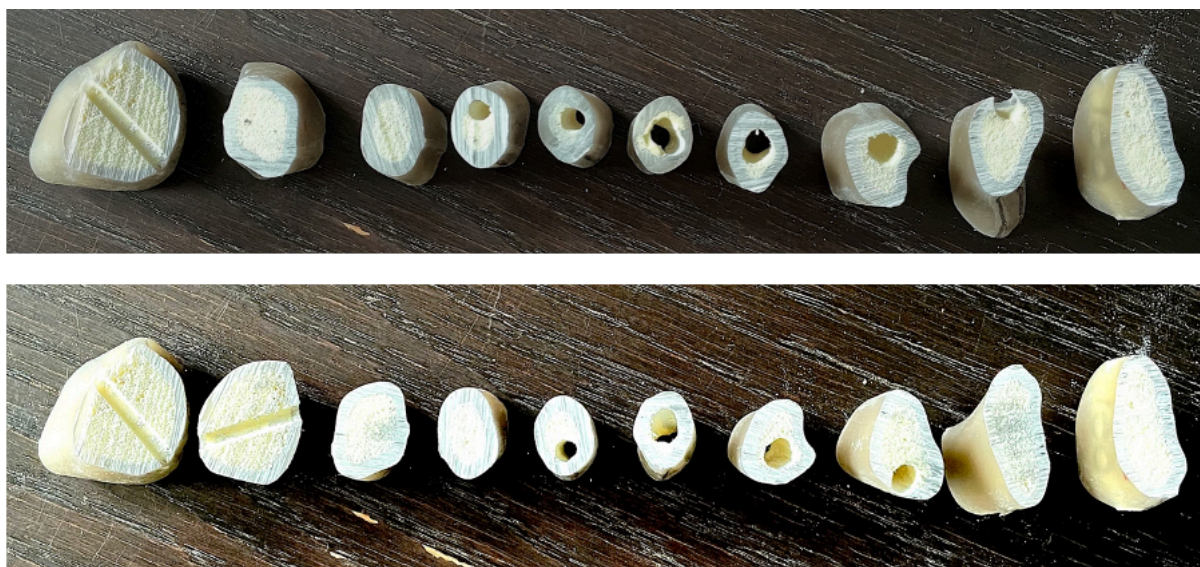
Figure 3. Highly variable shapes and sizes of the cross-sections of the same Sawbone®, viewed from both sides of the same section of the diaphysis, on the left is the sternal end. The holes are remnant of an intramedullary implant inserted from the acromial to the sternal end.
