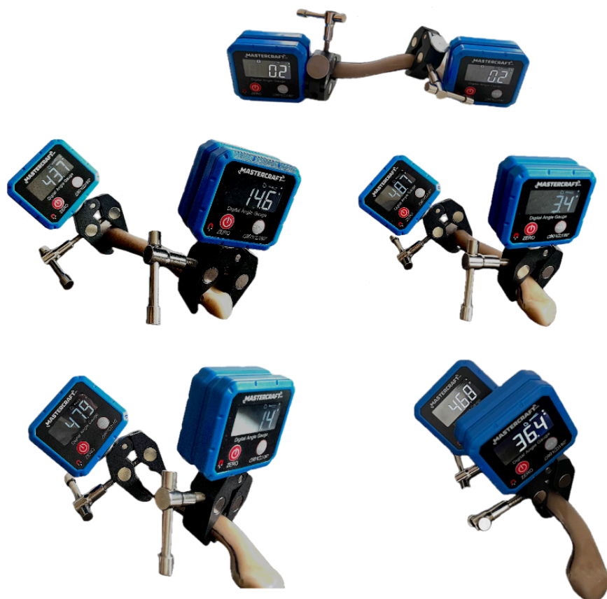
Figure 16. Measurement of the version angle and the sectional torsion angles at one-fifths' intervals from acromial to sternal end of a large left Sawbone®.
