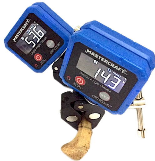
Figure 9. Digital goniometer devices are applied at the proximal and distal parts of the diaphysis of a cadaveric clavicle, which has a torsion angle of 39.3 degrees.
