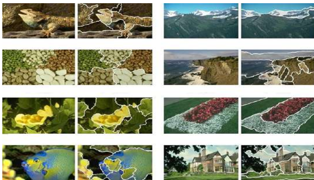
Figure 7. Segmentation results of some examples (one scale, size 192 *128 pixels).
