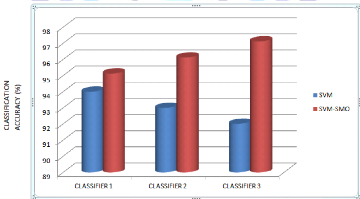
Figure 7 Comparative results showing the performance of classifiers during fault classification of power transformer.
