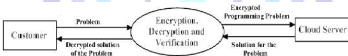
Figure 4: Level 0 Context Diagram for Dataflow of cloud system.
