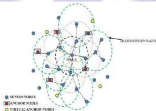
Figure 4: Localization using Virtual Anchor Nodes
