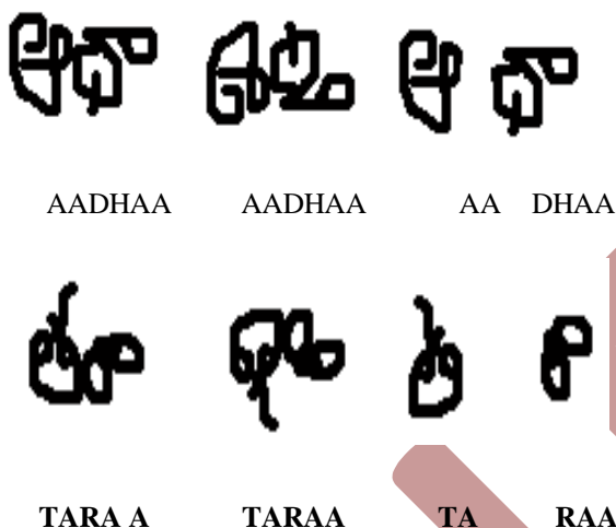
Fig.2. Segmentation of Touching Telugu Alphabets by using Bottom-Left drop fall from Left to Right and Top to Bottom
