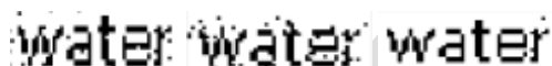
Fig 4.7: DCT based Extracted watermarks after applying Salt & pepper, Speckle & poisson attack respectively.
